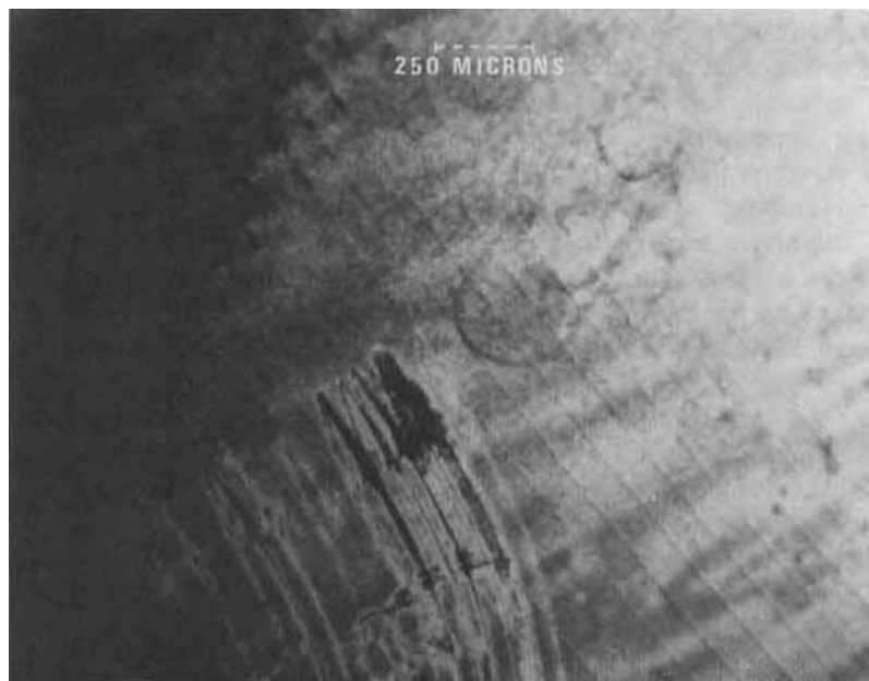
FIGURE 3 3 layer cadmium arachidate film with deliberately induced scratches.
