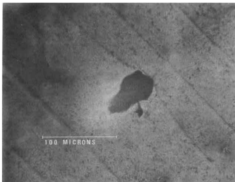
FIGURE 2 Photograph of a 3 layer cadmium arachidate film, showing a hole in the film.
