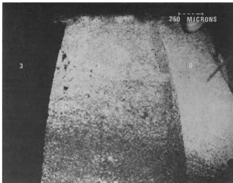
FIGURE 4 Photograph of 0, 1 and 3 layers of \omega -tricosenoic acid showing difference in alignment of the 1 and 3 layer regions.
